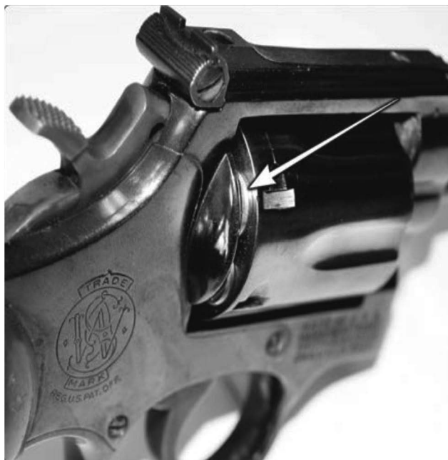
(Figure 6-2) Cylinder placement with partial load
